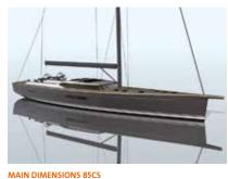
Length overall 25.82 m Length waterline 23.17 m Maximum beam 6.40 m
