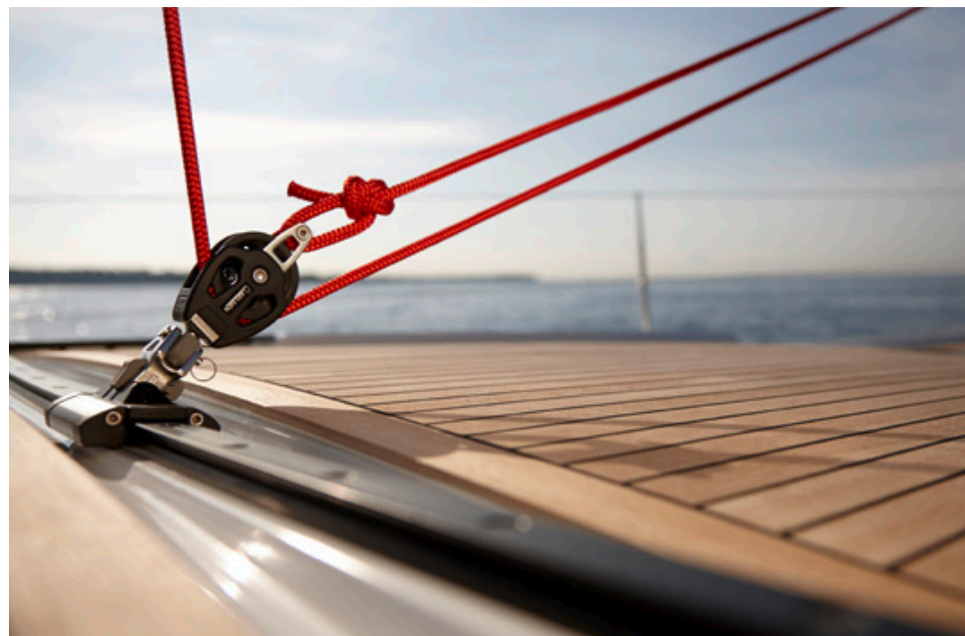
4 Integrated self-tacking jib track with „high-load“ slide system.
