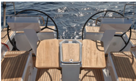
Double steering system, GRP wheels, black or white, Y spoke, 2 x 1000 mm
