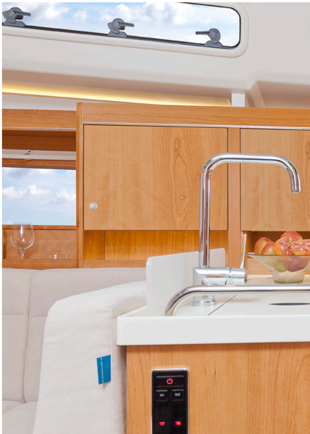
3 Galley in L-shape with 3-flame gas stove, oven and integrated double fridge (top and front loader).
