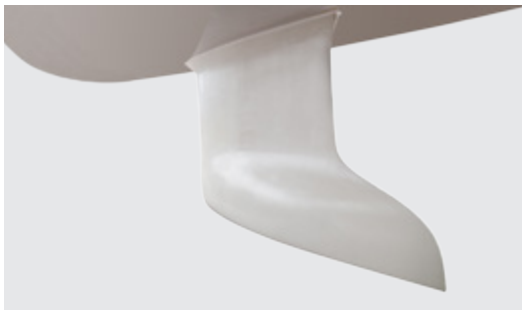
Shallow draft L-shape keel (1.82 m), cast iron
