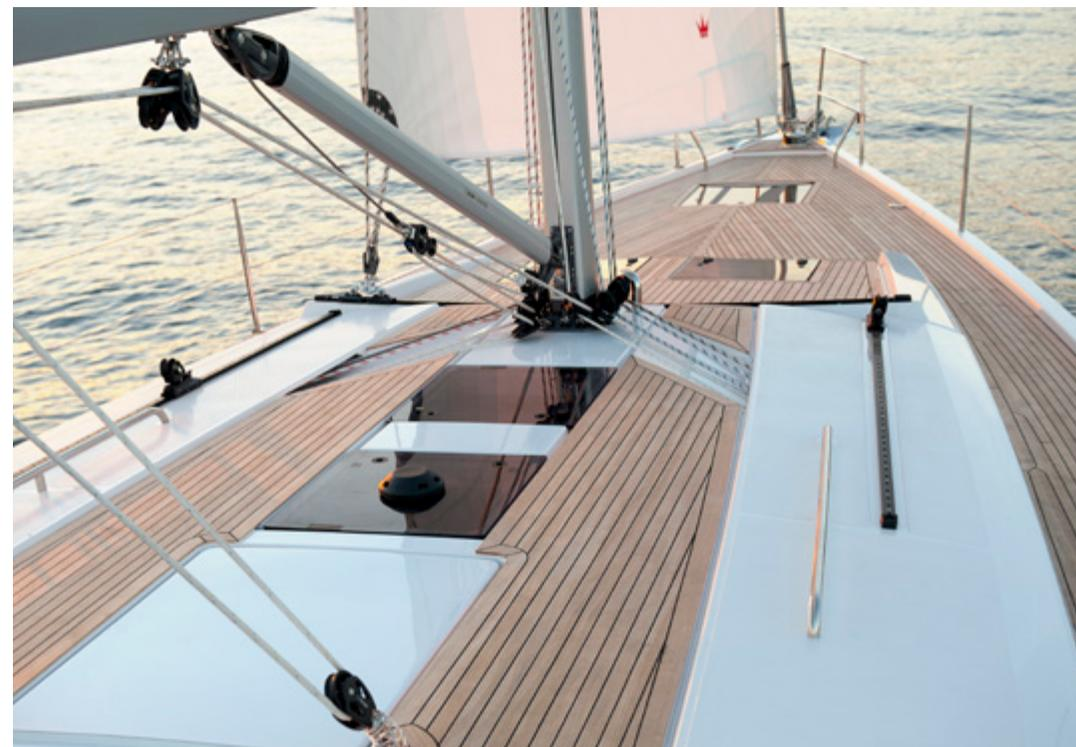
3 Consistent: Deck with flush hatches and hidden lines.
