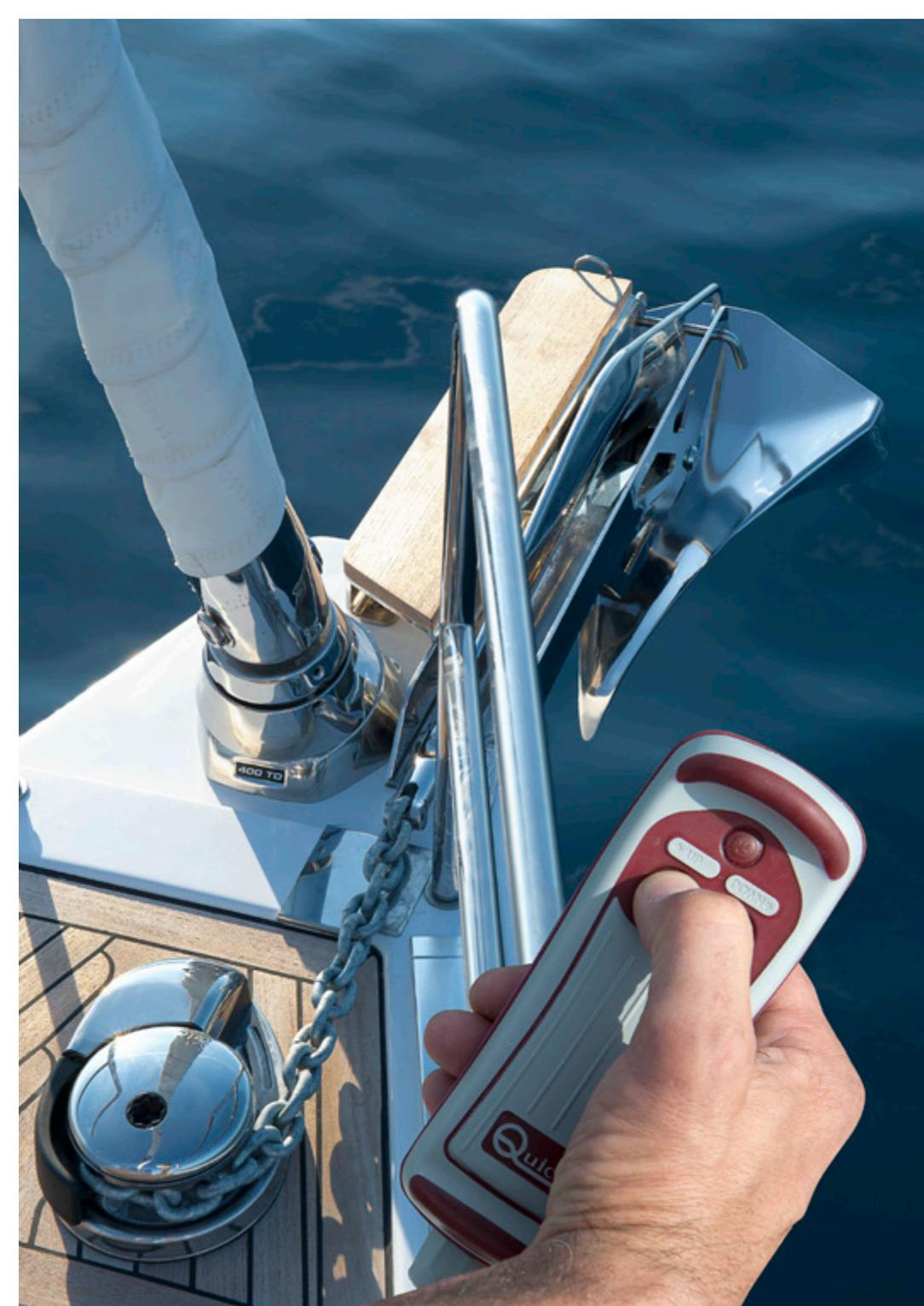
1 Laying anchor made easy: at the touch of a button on the remote control.
